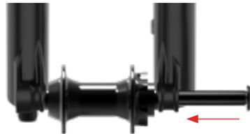
**⚠ WARNING:** Use hand pressure only. Never use any tool to tighten the 15QR levers onto the lower legs. Over-tightening the levers can damage the axle or fork dropouts, leading to a sudden failure with one or more of these components, resulting in **SERIOUS INJURY OR DEATH**.
