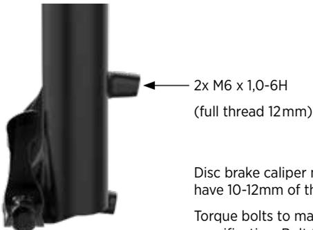
Disc brake caliper mount bolts must have 10-12mm of thread engagement.
