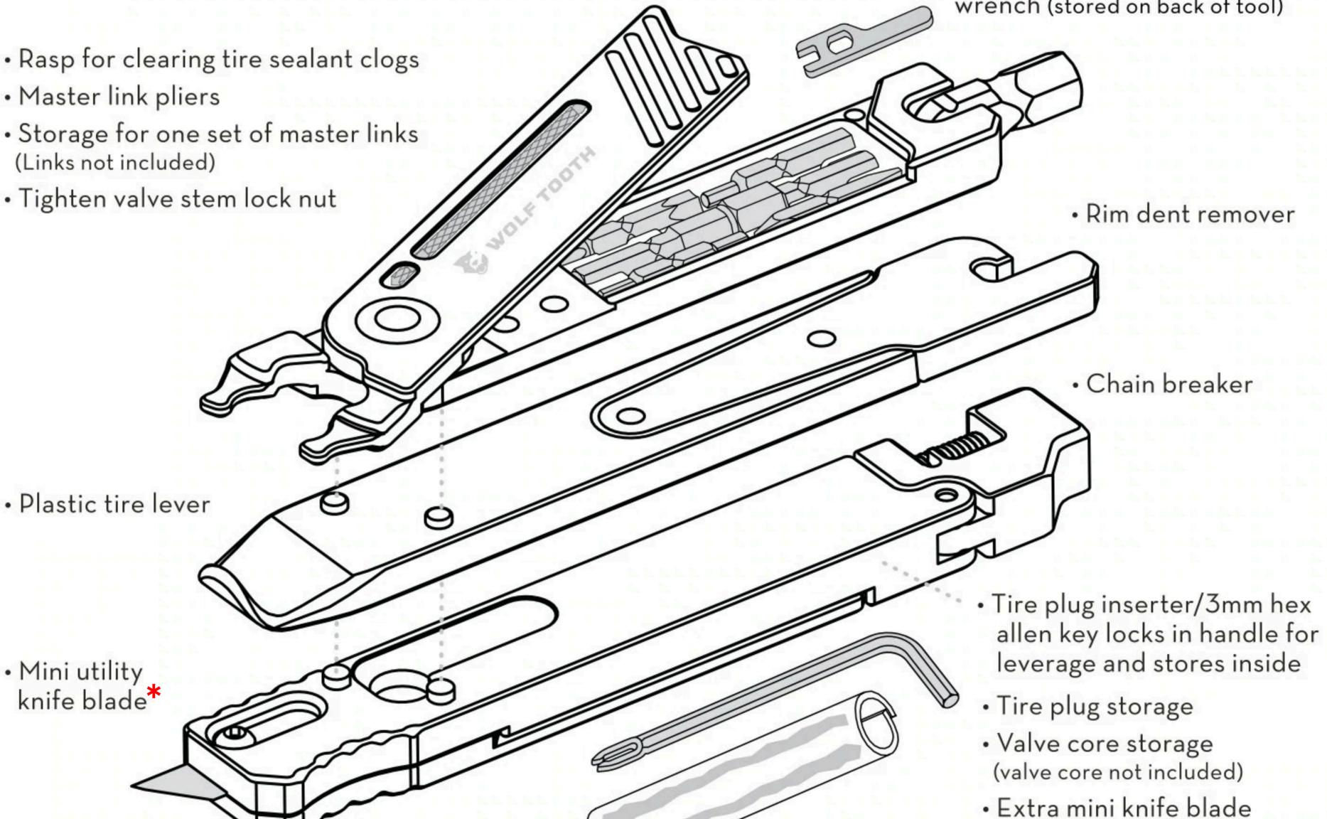
Multi-tools stack and attach to each other using magnets and pins
