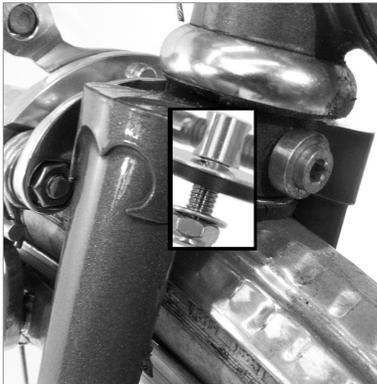
3. Re-tighten the brake bolt nut so the brake is reinstalled.
