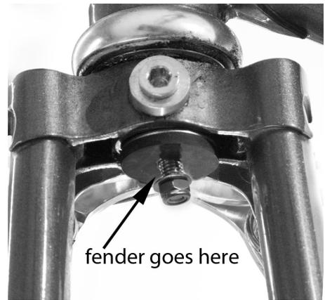
7. Since the fork crown on most bikes is not perfectly tangent to the wheel, you'll need to align the fender to the wheel. Simply hold the fender on either side of the fork crown and apply a little pressure to line it up with the wheel. This will make a little dent in the fender around the mounting screw and allows the fender to line up with the wheel.
