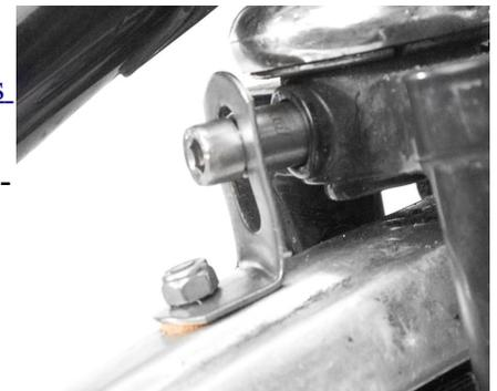
***Attaching the fender stays to the fork eyelets:***
