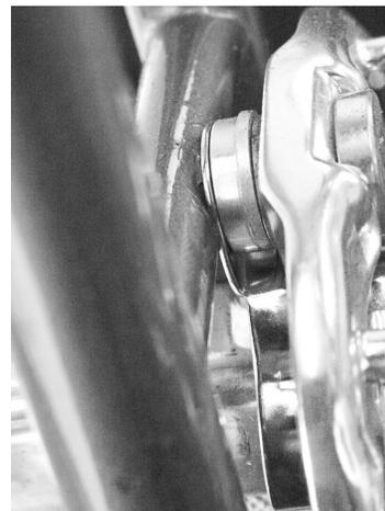
***Attach the fender stays to the rear eyelets:***
