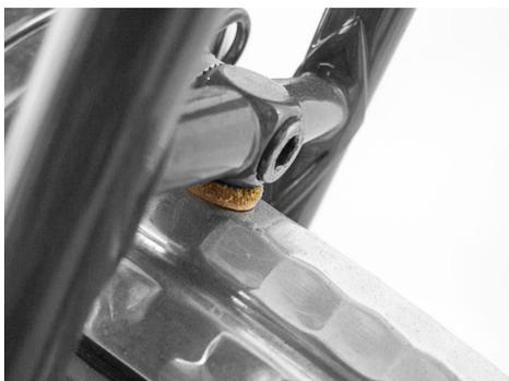
3. A few bikes don't have a hole in the seat stay bridge. In that case you can use a p-clamp to attach the fender.
