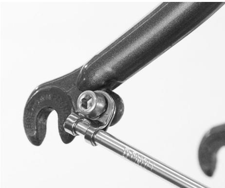
4. Tighten the R-clips and fork crown attachment.
