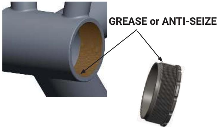
1. Apply grease or anti-seize to the frame & BB cup threads
