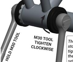
**2.** TURN THE RIGHT/DRIVE CUP UNTIL IT STOPS. With 2nd BB tool, hold the LEFT/NON-DRIVE Cup in place while you tighten the Drive cup fully. The 2nd tool gives you leverage so you feel when the Drive cup bottoms out on the Non-Drive cup.
